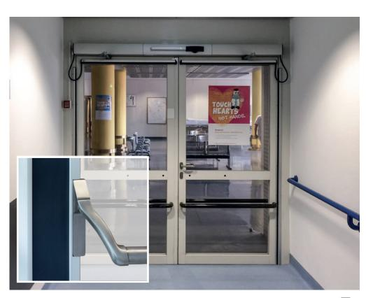
"Finger protection must not be installed on a fire or smoke protection door without the approval of the door manufacturer / system provider!"
