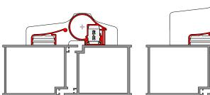
BA-28<sup>+</sup> with different surface mounted hinges
